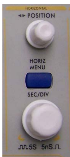
Fig. 10 Horizontal Control Zone
